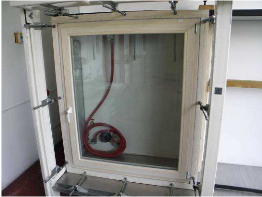
Picture 1 View of test specimen on window test rig Window closed
