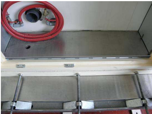
Picture 3 Rebate drainage
