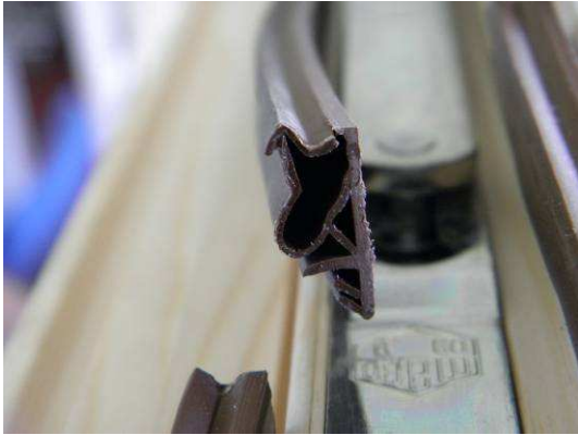
Picture 19 Centre seal
