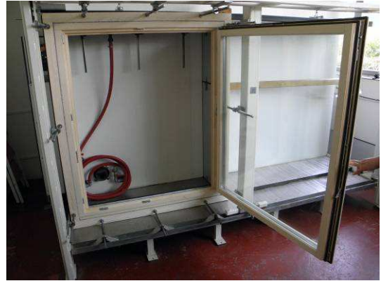
Picture 2 View of test specimen on window test rig Window open
