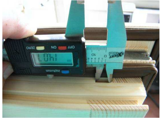
Picture 26 Vapour pressure equalisation
