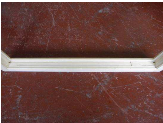
Picture 23 View of horizontal glazing rebate
